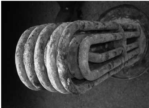
Fig 1. Heating element with scale deposits
